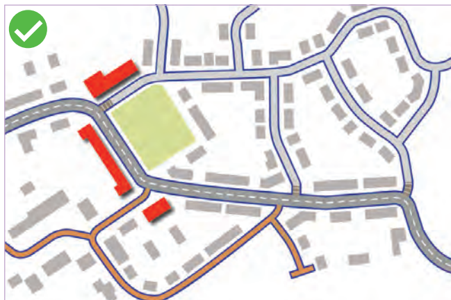
Revised layout: The street hierarchy is improved by realigning the main route and improving junction arrangements, street treatments and the location of community uses.
